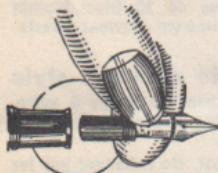
Remove old point by unscrewing to left (see illustration). Thread new point into pen by turning to right until it fits snugly. Remember, Esterbrook makes more than 30 different points so you can choose the point that is exactly right for you.
